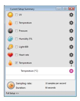
5. Click Full Setup, located at the bottom of the Current Setup Summary window to program the data logger's sample rate, number of samples, units of measurement, and other options
