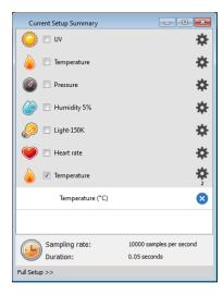
5. Click Full Setup, located at the bottom of the Current Setup Summary window to program the data logger's sample rate, number of samples, units of measurement, and other options
