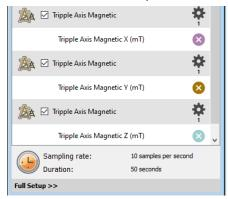
6. Click Full Setup, located at the bottom of the Current Setup Summary window to program the data logger's sample rate, number of samples, units of measurement, and other options
